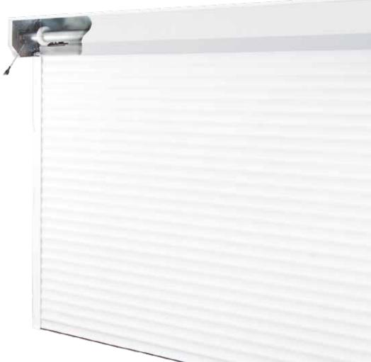
Gliderol Insulated Roller Doors take up very little space inside your garage. The standard configuration, using 77mm foam filled lath (Also available as a manually operated system), requires 300mm of headroom and is supplied with 70 or 90mm guides depending on specification. The compact version, using 55mm foam filled lath, requires only 205mm of headroom and is supplied with 65mm guides.
